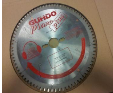
2.1 Circular saw blade: n. 80 teeth, 250 mm diameter, 32 mm hole diameter, n. 8000 rpm max
